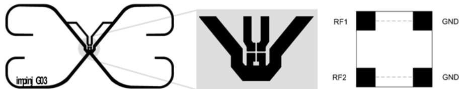
Figure 3-5 Two single-ended connections established for dual dipole antenna. Impinj Jumping Jack tag antenna shown (L) with antenna trace detail (C) and corresponding chip/antenna connections (R).
