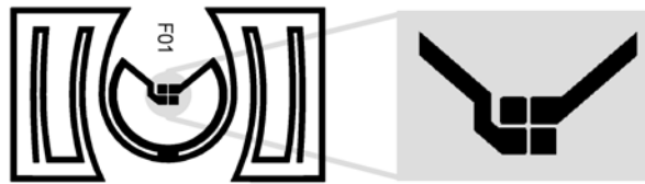
Figure 3-2 Antenna designed for single-ended connection. Satellite antenna shown (L), with antenna trace connection detail (R). Note the diagonal pad contacts between RF1 and GND.
